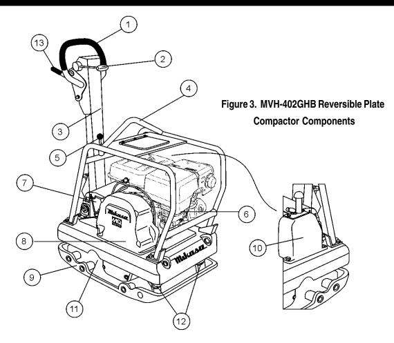
Figure 3 illustrates the location of the major components for the MVH-402GHB Reversible Plate Compactor. The function of each component is described below:
